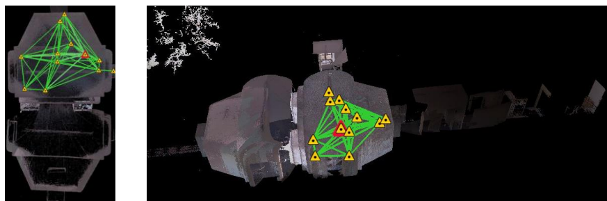
Fig. 6: 3D digital image and connector of interior image capture positions in floor plan and tilt angle
