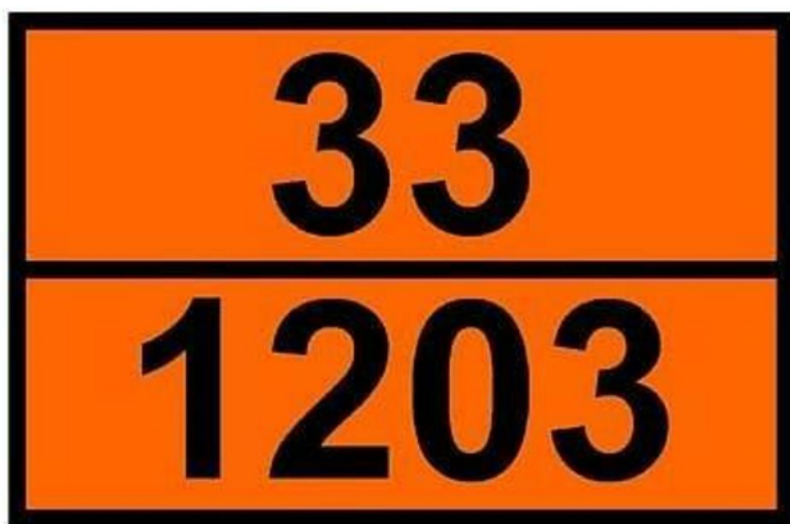
Figure 1 Kemler and UN code, Source: [10]
