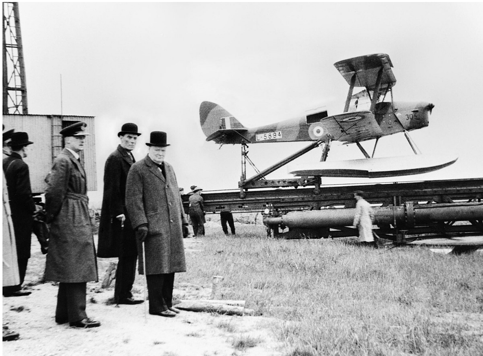
Obr. č. 6 - De Havilland DH.82B Queen Bee, start z katapultu, (dostupné z: https://commons.wikimedia.org/wiki/File:Winston_Churchill_and_the_Secretary_of_State_for_War_waiting_to_see_the_launch_of_a_de_Havilland_Queen_Bee_radio-controlled_target_drone,_6_June_1941._H10307.jpg )
